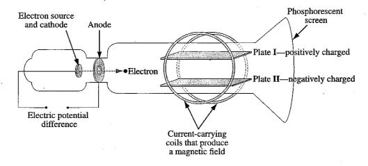
Electrons then pass undeflected through a region in which there is both an electric and a magnetic field. The electric field is produced between plate I and plate II, which are 3.00 cm apart. The electric potential difference between the plates is 12.0 V. Two current-carrying coils produce a magnetic field that is perpendicular to the electric field.
