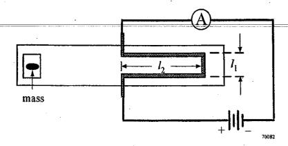
The diagram shows a current balance loop that includes the conductor where the length of segment  $l_2 = 8.60$  cm. A student places this current balance loop in a solenoid where the
